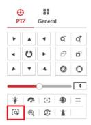
**b.** Click this button, when there are multiple targets detected by panoramic camera, select one target and left click its rule box, the PTZ camera will start to track that target.
