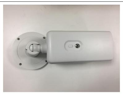
**Step4:** Unscrewing the screws to adjust the lens angle in order to adjust the image to the required monitoring site.
