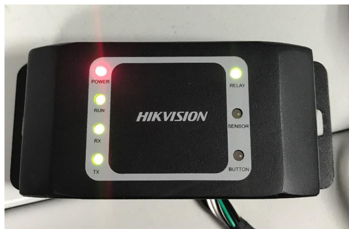
Figure 7, Secure Door Module availability – lights displayed
