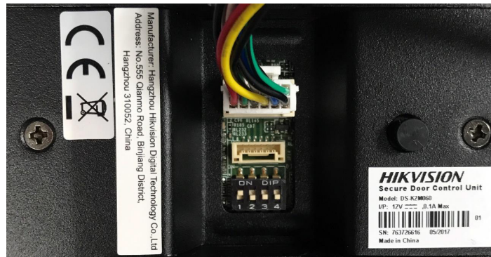
Figure 1, DIP switch settings
