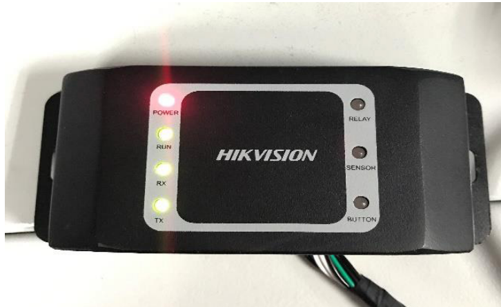
Figure 3, Operation lights on Secure Door Module
