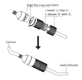
Figure 42, Waterproof Accessory Installation
