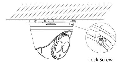
Figure 10, Loosen Lock Screw
