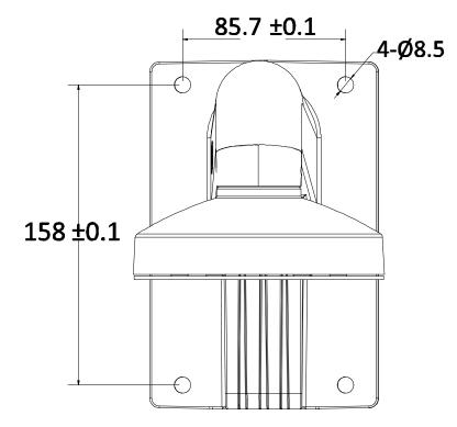
Figure 34, Dimensions of Typical Wall Mounting Bracket
