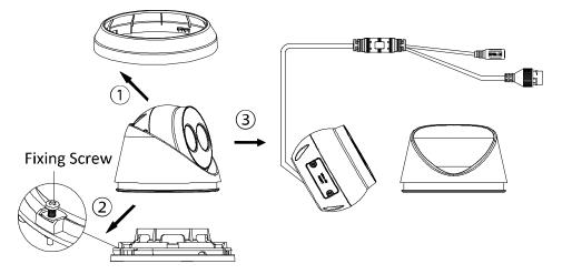
Figure 27, Disassemble the Camera
