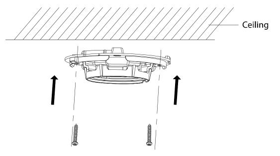
Figure 16, Secure the Camera to the Ceiling
