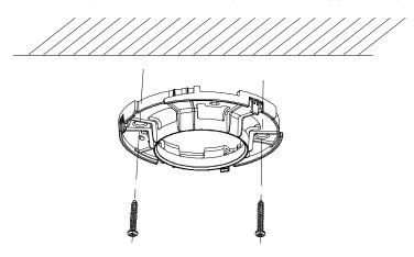
Figure 23, Fix Mounting Base to Ceiling
