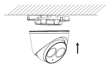
Figure 24, Install the Camera
