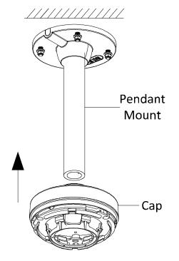
Figure 39, Install the Cap
