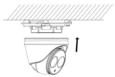
Figure 9, Secure the Camera to the Mounting Base
