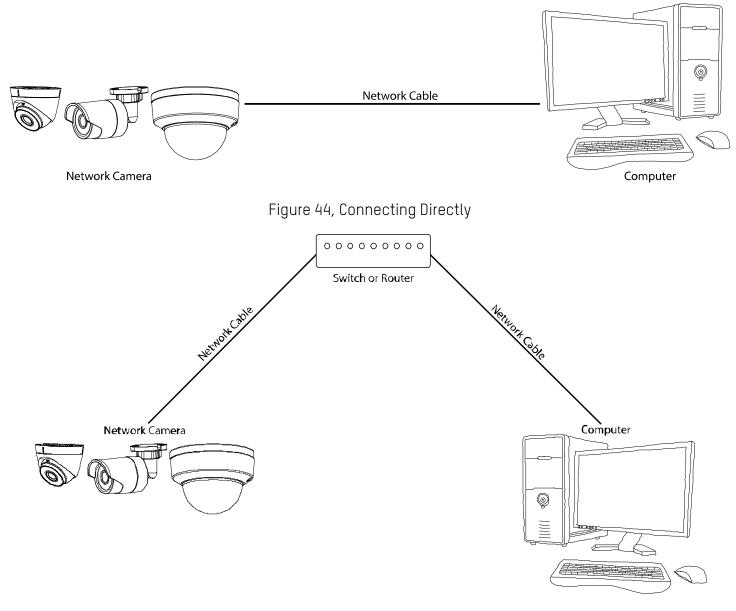
Figure 45, Connecting via a Switch or a Router
