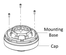
Figure 38, Fix Mounting Base
