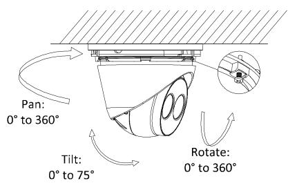
Figure 32, Adjust Surveillance Angle
