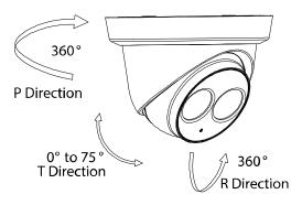
Figure 25, Adjust the Lens
