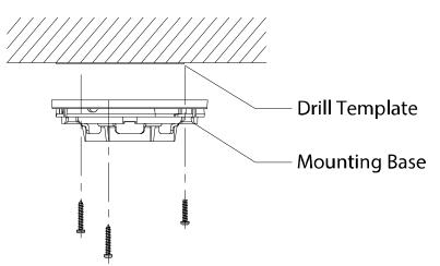
Figure 30, Fix Mounting Base
