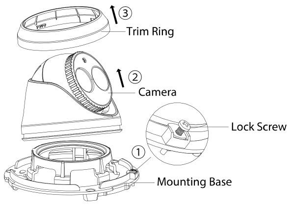
Figure 5, Disassemble the Camera
