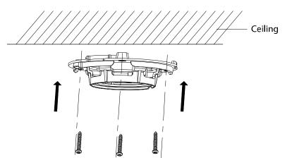
Figure 8, Secure the Mounting to the Ceiling
