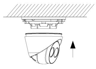
Figure 31, Install the Camera
