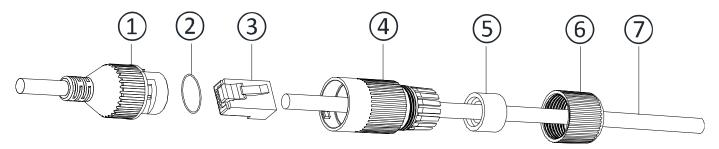
Figure 41, Waterproof Accessory Components
