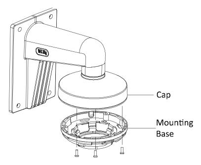
Figure 35, Fix Mounting Base
