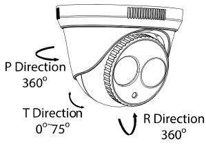
Figure 17, Adjust the Lens
