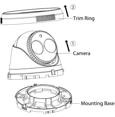
Figure 13, Disassemble the Camera
