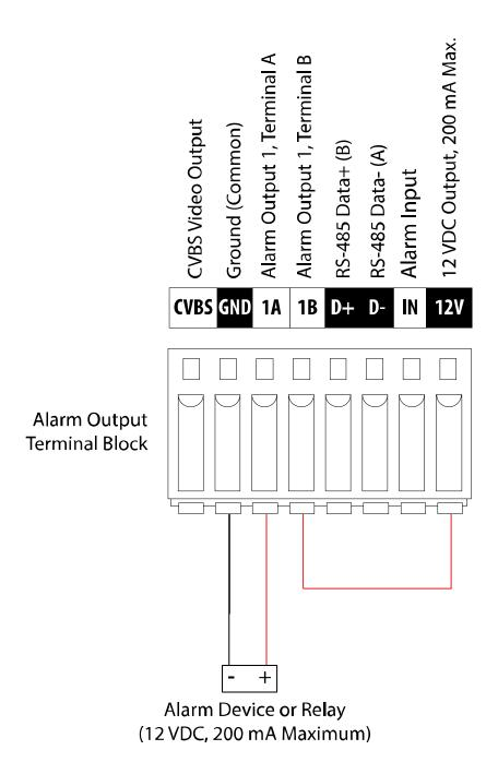
Alarm Output with Power from Camera
