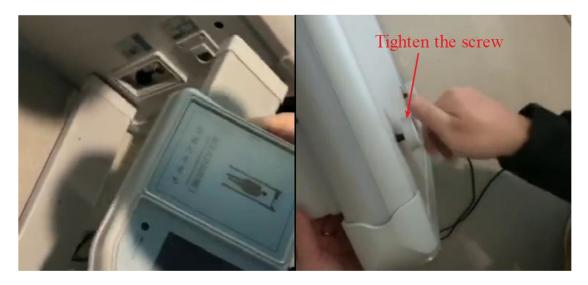
2) After connecting the door panels, connect the cable. The right side will be the power cable and signal cable, the left side will be the signal cable only. Pay close attention to the left and right signs, and make sure the correct cables are connected to each side.
