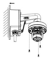
Figure 22, Fix the Camera to Wall Mounting Bracket
