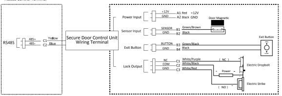
Note: The external power supply and the secure door control terminal should use the same GND cable.
