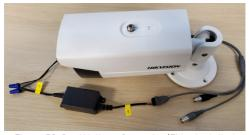
Figure 52, Dual Voltage Converter/Filter Installed
