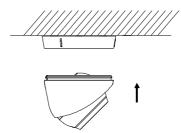
Figure 28, Secure Camera with Mounting Base
