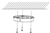
Figure 27, Attach Mounting Base to Ceiling
