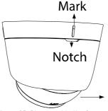
Figure 25, Disassemble the Camera
