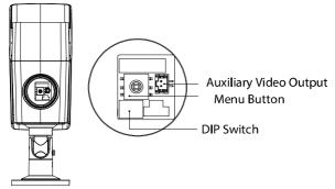
Figure 21, Internal Interface and Button
