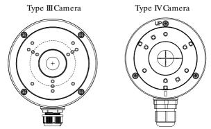
Figure 23, Install Junction Box
