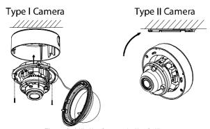
Figure 9, Affix the Camera to the Ceiling
