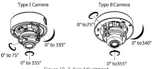
Figure 10, 3-Axis Adjustment
