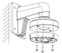
Figure 33, Attach Mounting Base to Bracket
