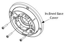
Figure 35, Install Turret Camera Mounting Base
