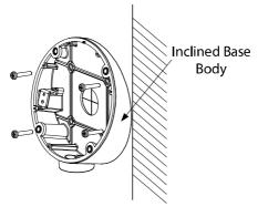
Figure 36, Affix Inclined Base Body
