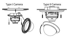
Figure 8, Fix the Camera to the Mount
