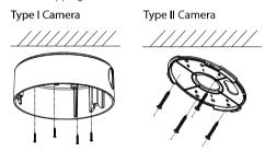
Figure 4, Attach the Back Box/Base Plate
