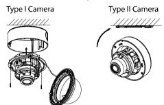
Figure 5, Affix the Camera to the Ceiling
