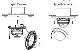
Figure 10, Secure the Camera
