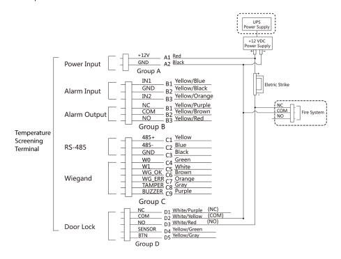
Figure 16, Device Wiring
