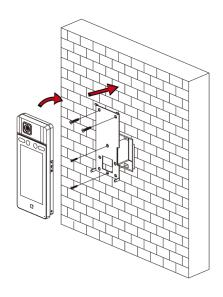
Figure 2, Install Device
