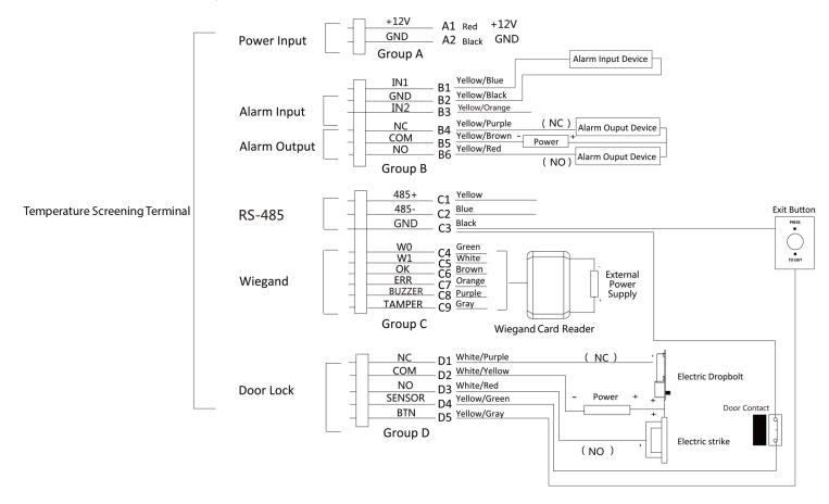
Figure 10, Device Wiring
