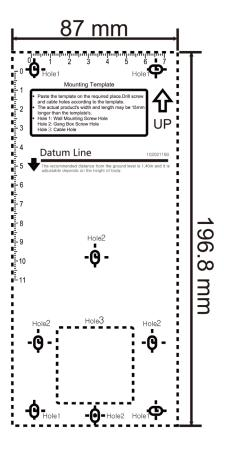
Figure 4, Mounting Template
