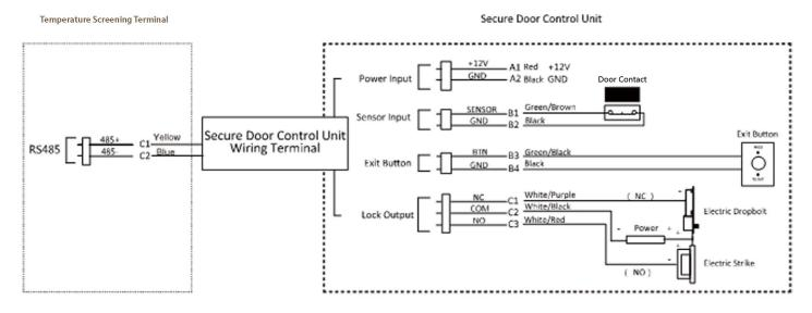
Figure 11, Secure Door Control Unit Wiring
