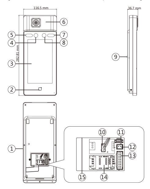
Figure 1, Temperature Screening Terminal Diagram
