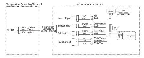
Figure 17, Wiring Diagram
