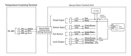
Figure 15, Wiring Secure Door Control Unit
