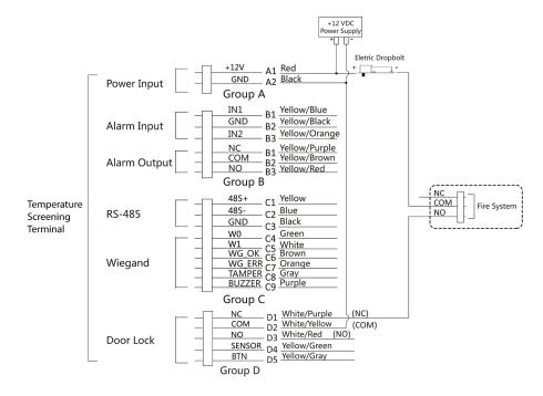
Figure 14, Wiring Device
