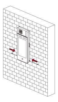
Figure 8, Secure Device
