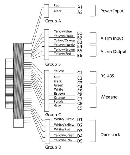
Figure 9, Terminal Diagram
