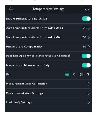
Figure 27, Temperature Measurement Parameters
