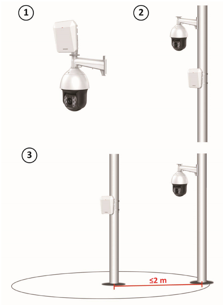
Figure 5-5 Installation Scene for One-Point Calibration
