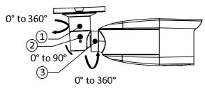
Figure 2-3 3-Axis Adjustment
