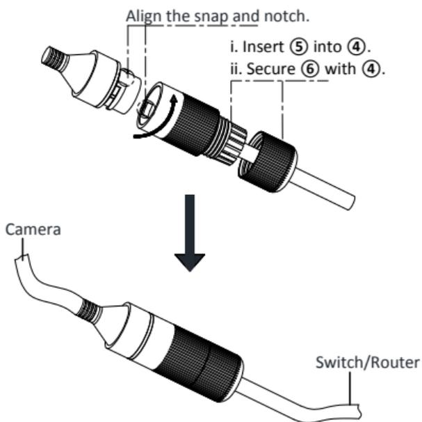
Figure 2-16 Waterproof Accessory Installation
