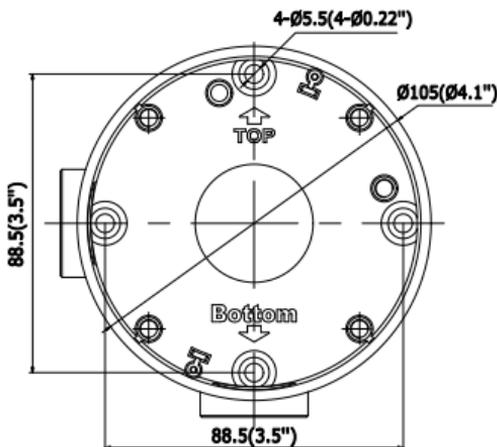
Figure 2-7 Dimension of Junction Box
