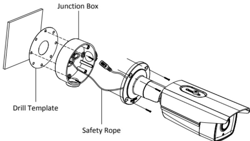
Figure 2-8 Installation with a Junction Box
