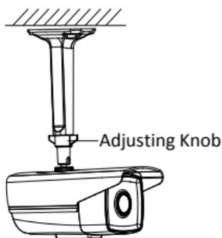
Figure 2-13 Install the Camera
