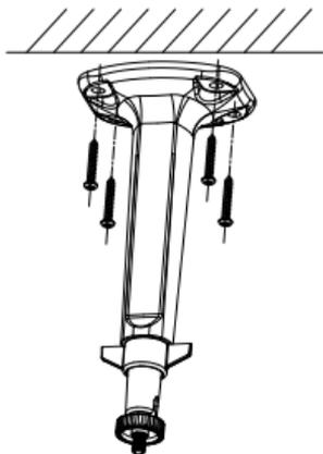
Figure 2-12 Fix the Bracket
