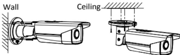
Figure 2-4 Install the Camera
