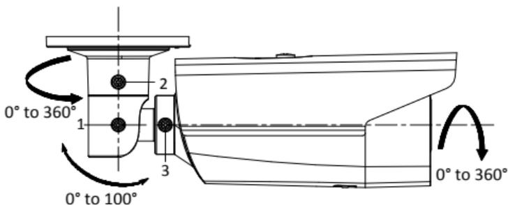
Figure 2-5 Adjust the Surveillance Angle
