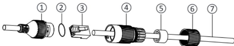
Figure 2-15 Waterproof Accessory Components
