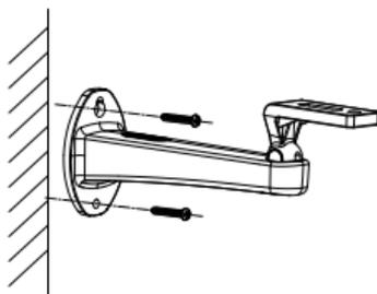
Figure 2-10 Fix the Bracket
