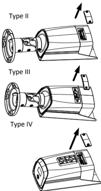
Figure 2-1 Expose Memory Card Slot
