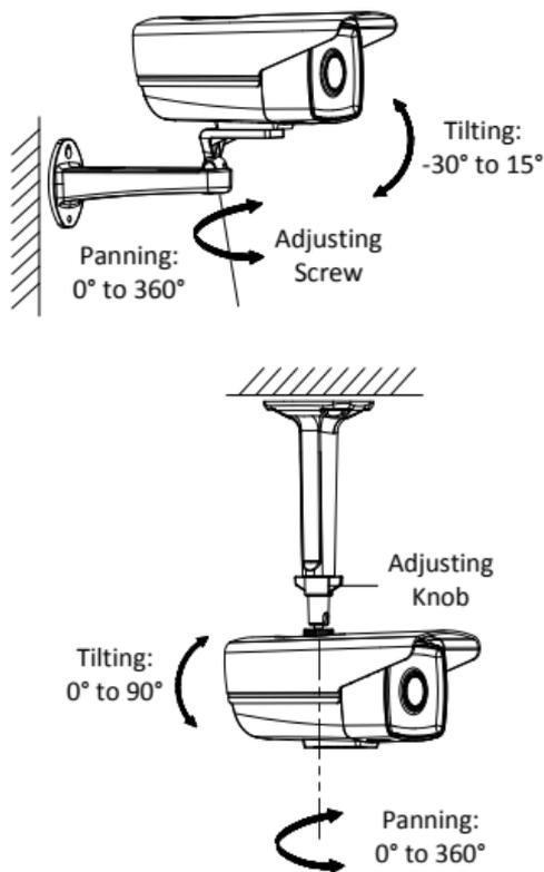
Figure 2-14 Adjust the Angle
