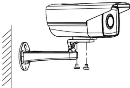
Figure 2-11 Install the Camera
