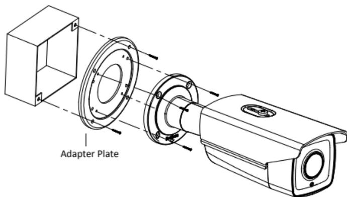
Figure 2-9 Installation with a Gang Box
