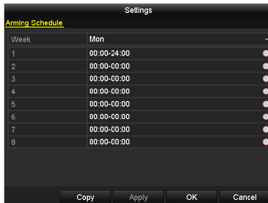
Figure 153, Set Arming Schedule of Alarm Output
