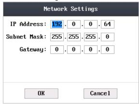
3. Modify network parameters of the device, including IP address, subnet mask, and gateway address.
