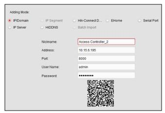
4. Edit the device information, including the adding mode, the device name, the device IP address, port No., user name, and the password.
