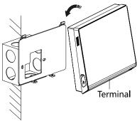
5. Tigten the srews to fix the terminal on the mounting plate and complete the installation.
