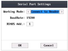
3. Modify parameters of the serial port, including working mode, Baud Rate, and RS-485 address.
