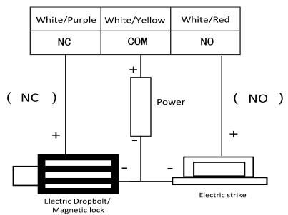
**Note:** Signal input interface of the door status (DOOR\_NC, DOOR\_COM, DOOR\_NO) is used to recognize whether the door is locked. If the NC interface is connected for opening door, the NO interface can only be connected for locking door.
