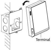
5. Tigten the srew to fix the terminal on the mounting plate and complete the installation.
