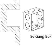
2. Secure the device mounting plate on the gang box with two srews (supplied).
