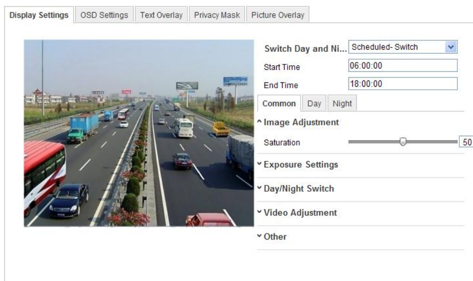
Figure 6-37 Day/Night Scheduled-Switch Configuration Interface
