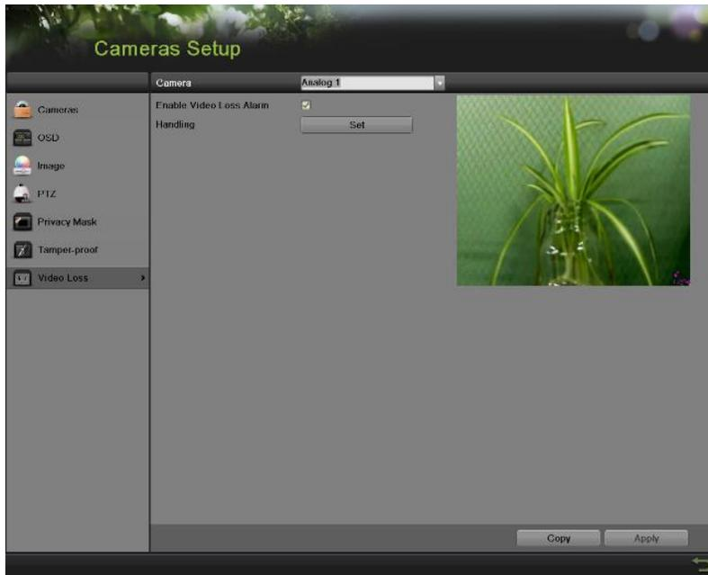
Figure 129 Video Loss Detection Menu
