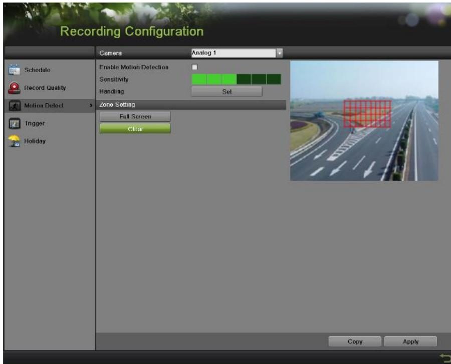
Figure 115 Motion Detection Settings Menu
