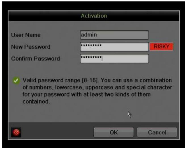
Figure 14 Risky (Inadequate) Strength Password
