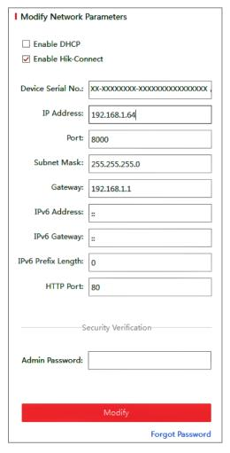
Figure 42, Modify the IP Address
