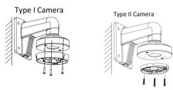
Figure 20 Install Mounting Base to the Bracket
