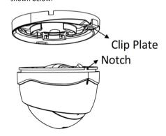
Figure 12 Disassemble the Camera
