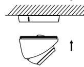
Figure 6 Secure the Camera with Mounting Base
