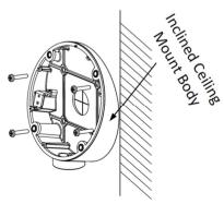
Figure 10 Fix the Inclined Base Body
