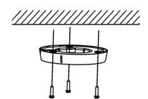
Figure 5 Attach the Mounting Base to the Ceiling
