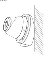
Figure 11 Fix the Camera to the Inclined Base
