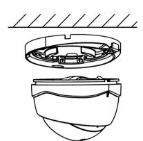
Figure 15 Secure the Camera
