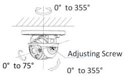
Figure 20 Type I Camera 2-Axis Adjustment
