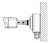
Figure 10 Fix Junction Box Cover to its Body
