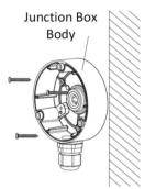
Figure 9 Fix the Junction Box to the Wall/Ceiling
