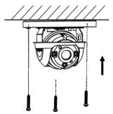
Figure 19 Fix the Mounting Base
