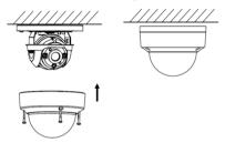
Figure 21 Bubble Reinstallation
