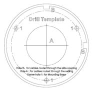
Figure 7 Junction Box Drill Template
