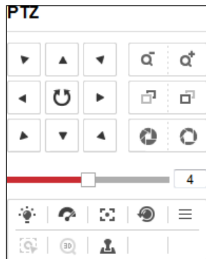
Figure 30, PTZ Control Panel
