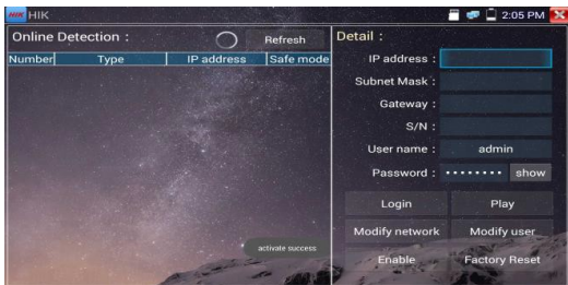
Figure 142, Camera IP Modification Screen
