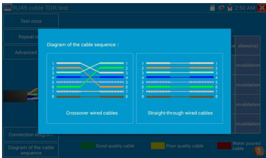
Figure 111, Cable Sequencing Diagram
