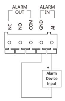
Figure 2-5 Alarm Device Input Wiring
