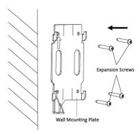
Figure 3-2 Install the Plate
