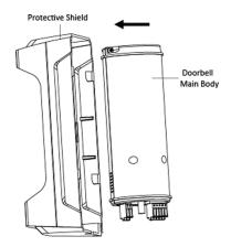
Figure 3-4 Fix the Body to the Shield
