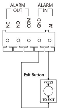
Figure 2-4 Exit Button Wiring
