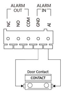
Figure 2-3 Door Contact Wiring
