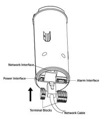
Figure 3-3 Insert Terminals and Network Cable
