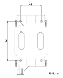
Figure 3-1 Wall Mounting Plate
