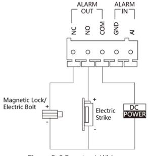
Figure 2-2 Door Lock Wiring
