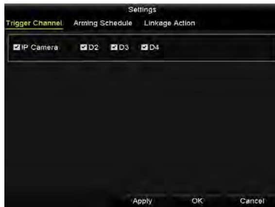
Figure 86, Set Trigger Camera of VCA Alarm
