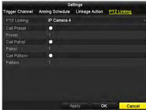
Figure 140, Set PTZ Linking of Alarm Input
