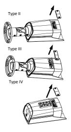
Figure 2-1 Expose Memory Card Slot
