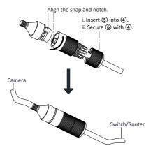
Figure 2-16 Waterproof Accessory Installation
