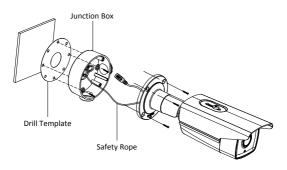
Figure 2-8 Installation with a Junction Box
