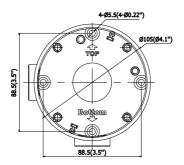
Figure 2-7 Dimension of Junction Box
