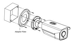
Figure 2-9 Installation with a Gang Box
