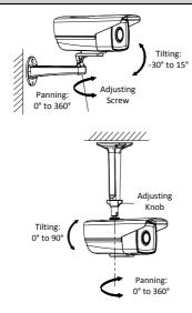
Figure 2-14 Adjust the Angle
