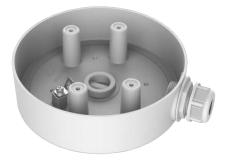
The junction box should be installed on a flat surface. Waterproof rubber is necessary for outdoor application. The wall must be capable of supporting at least three times the total weight of the camera and bracket. The maximum load capacity of the junction box is 11 lbs (5 kg).
