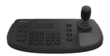
The Hikvision DS-1200KI network keyboard is a 4-axis joystick control device. It supports Multi-Functional Video Center (MVC) and Matrix Access Gateway (VAG) access, as well as PTZ control and picture capture.
