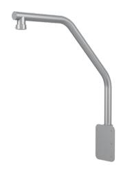
The mount should be installed on a flat surface. Waterproof rubber is necessary for outdoor application. The wall must be capable of supporting at least three times as much as the total weight of the camera and the mount. The mount's maximum load capacity is 22 lbs (10 kg).
